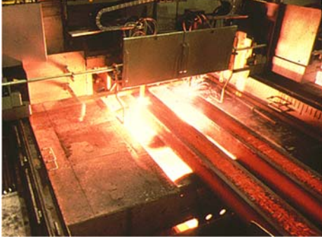
Steel Ingots being rolled
